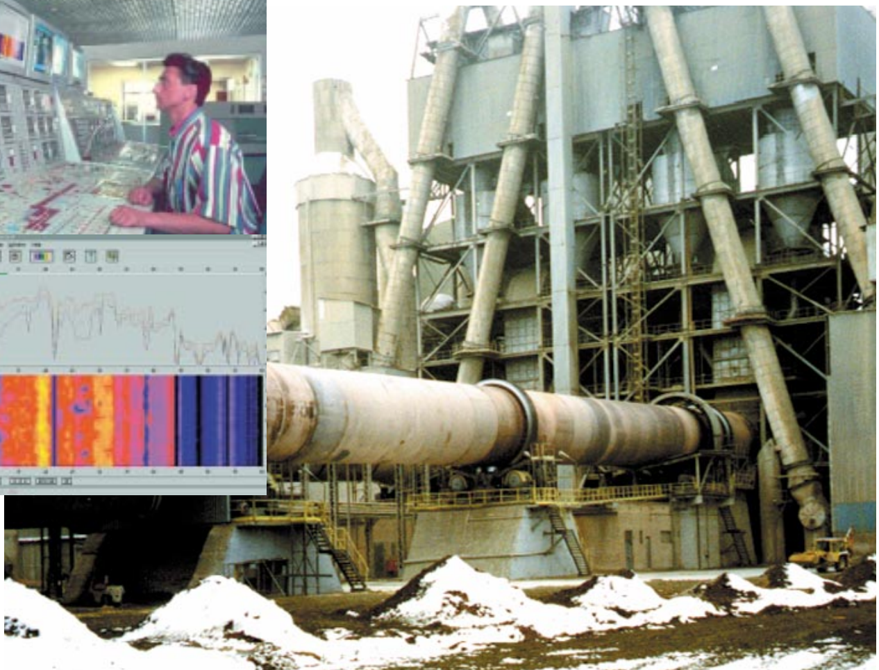
The CS100 System provides real time kiln shell temperature analysis.
